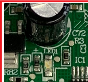
LED1: Drive failure indicator
