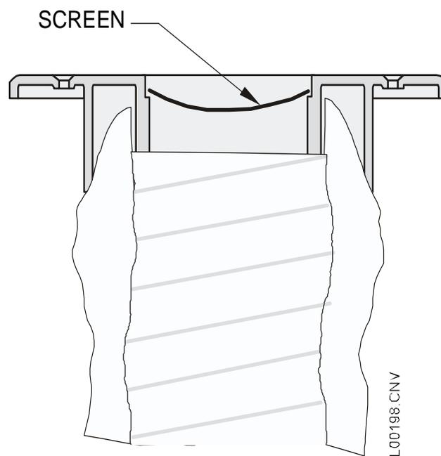
Figure 2. Installation of Outlet Screen
