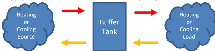
A buffer tank can **never** be used for backup heat. Electric heating elements may be installed in a buffer tank only for *\*emergency\** heat. If so, a TPV and element thermostat set at max 120F is required.
