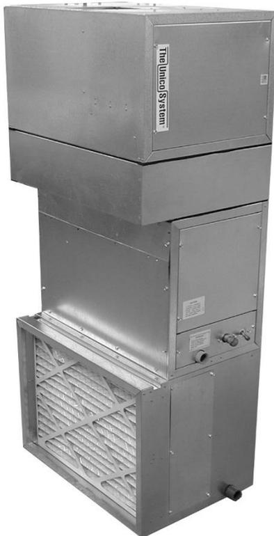
Cabinet construction is galvanized steel and fully insulated. The Unico System cooling module uses a thick copper tube/aluminum fin coil that produces superior moisture removal compared to a more conventional system. It comes standard with a corrosion resistant primary drain pan. The refrigerant coil module includes a thermostatic expansion valve and freeze protection controls for proper operation and to prevent icing. Water coils are equipped with a drain and a vent valve.
